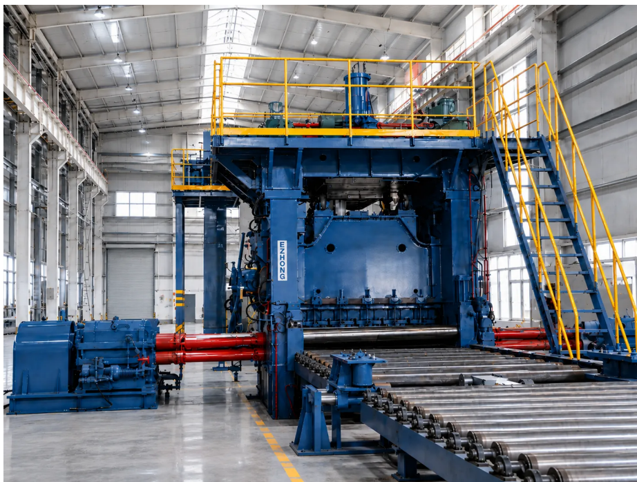
Baowu | EZW43CY-12×2200 for armor plate leveling.
