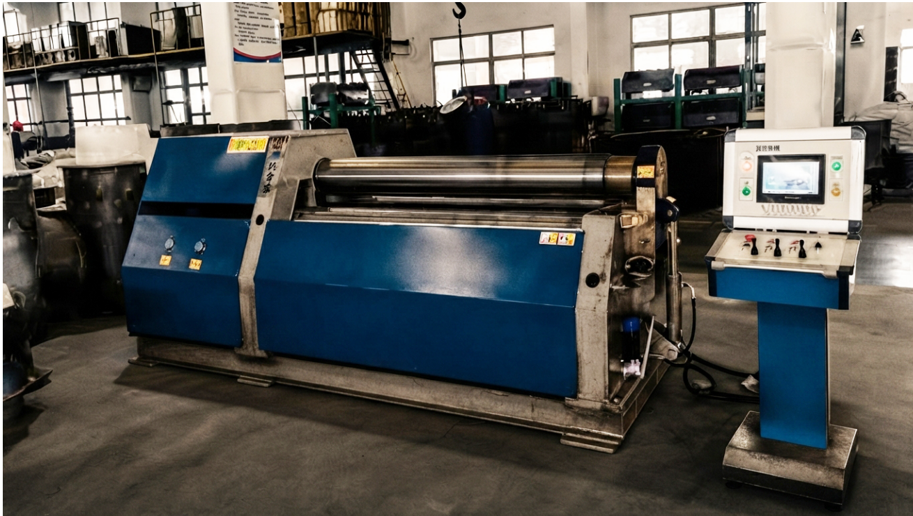
EZHONG 4-roll plate rolling machine with a separate control console.
