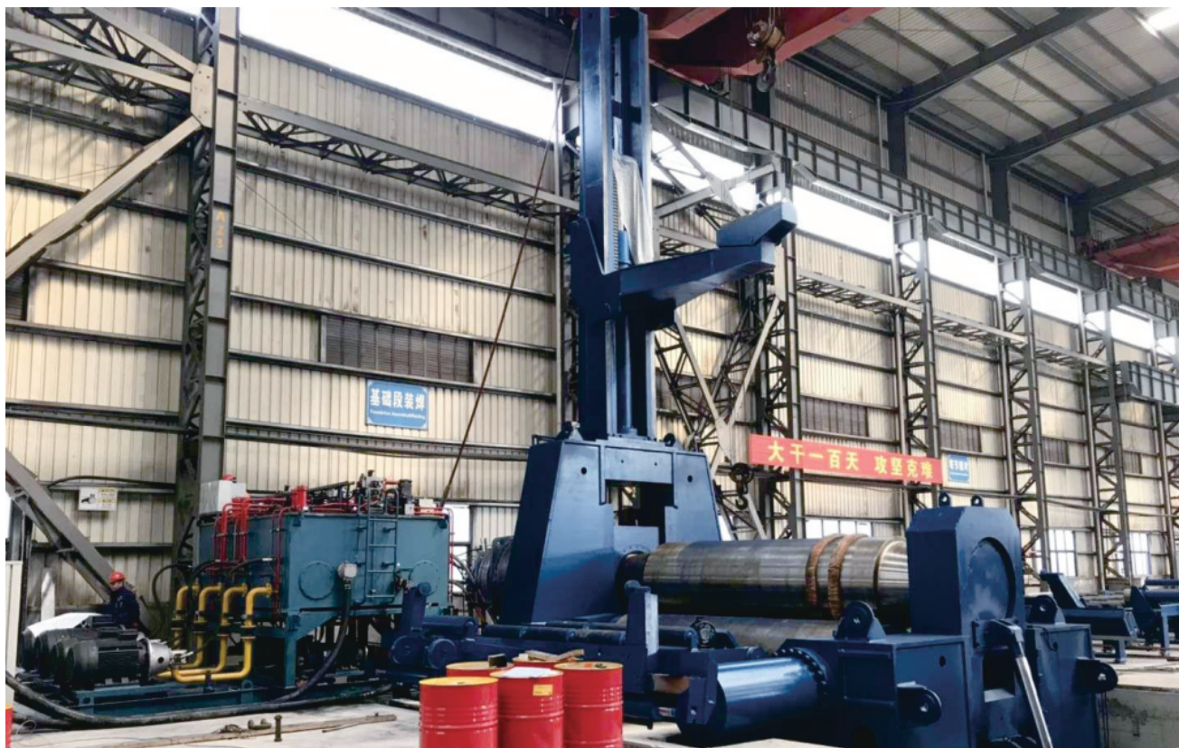
EZW11S-180×3500 | Plate rolling machine with overhead support.
