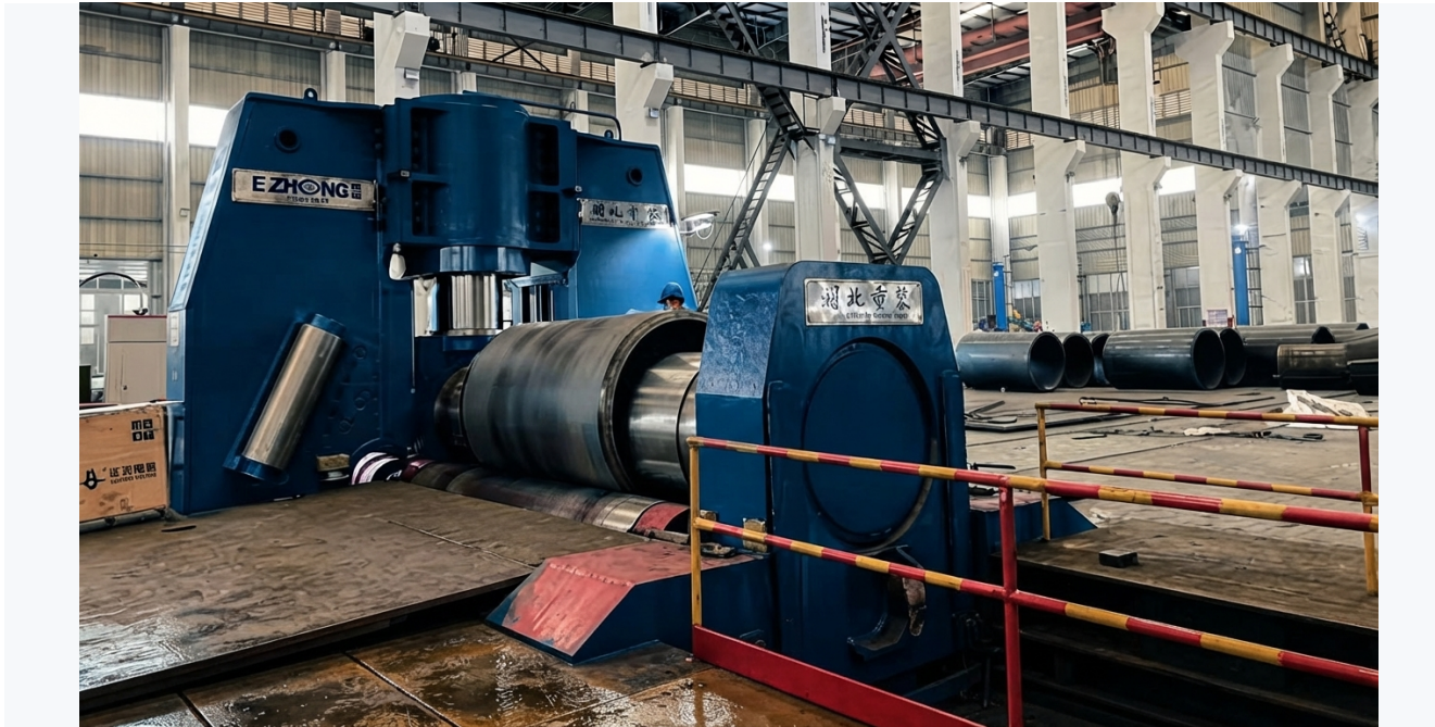
Heavy-duty plate rolling machine with dual-motor drive.
