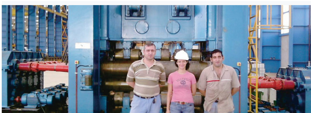
W43-60×2500 | 9-roll plate leveler installed in Afghanistan.
